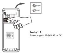
Before using the device for the first time, turn on the device, press and hold the reset button for approximately 5 seconds until "System reset" is heard and then release the button.
