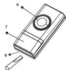
The doorbell operates at a frequency of 433MHz. The range is maximum 200m in an open area. The batteries for the receiver are alkaline 1.5V (LR03, AAA). The battery for the transmitter is alkaline 12V (LR23A).
