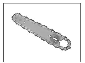
**2.** Remove the guide bar and replace the chain. Align the inner links of the chain into the groove of the guide plate.
