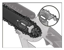
**3**. Place the chain around the sprocket and make sure the plate is straight and the chain is not slanted.
