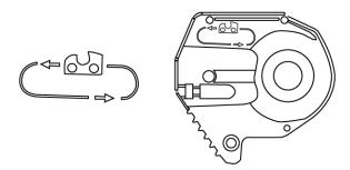
4. Replace the side cover and tighten the lock nut
