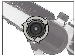
**1**.Unscrew the wing nut and remove the cover.
