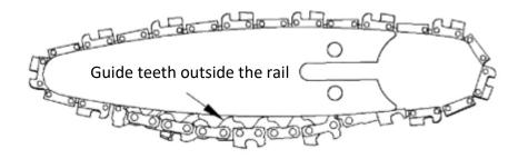
Grasp the tooth in the middle of the guide rail and pull it downwards. If a total of 3 teeth are exposed, the chain is correctly tensioned. Depending on the situation, either tighten or loosen the chain.
